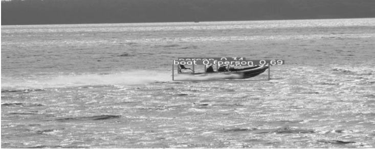
Fig.1. YOLO5 Small for the detection and tracking of a moving motorboat and people
